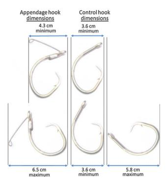
Fig. 2 14/0 circle hook with appendage and standard control 14/0 circle hook
