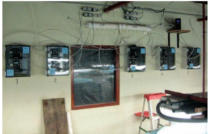
Figure 5. Gas-flow controllers and manifolds used for mixing and distribution of air and CO 2 . Photo: Donald Bromhead
