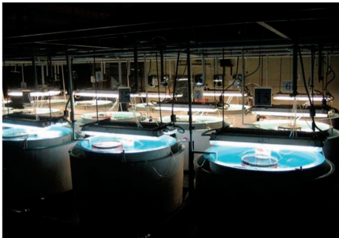
Figure 6. Multiple experimental tanks with nested egg incubators. Photo: Donald Bromhead
