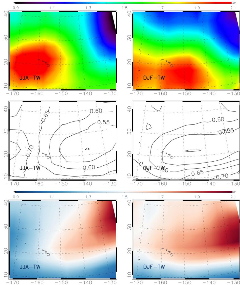
**Fig. 9.** Six year median value of the (top row) MBL height (km); (middle row) standard deviation of MBL height (km); and (bottom row) relative minimum gradient (RMG), per  $5^\circ \times 5^\circ$  grid under trade wind conditions for JJA-TW (left) and DJF-TW (right).
