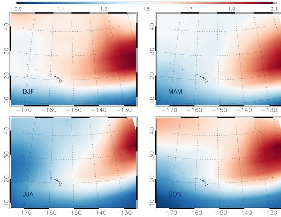
**Fig. 8.** Horizontal distribution of inversion strength, estimated by the relative minimum gradient (RMG). The RMG is calculated per  $5^\circ \times 5^\circ$  grid, for DJF (top left), MAM (top right), JJA (bottom left), and SON (bottom right).
