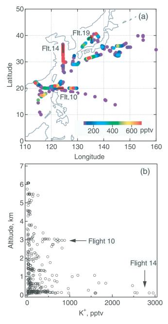
**Figure 6.** (a) Spatial distribution and (b) vertical distribution of water-soluble fine-particle potassium measured on the NASA P-3B aircraft in the western Pacific during TRACE-P. The locations of three specific plumes discussed in detail are also shown in Figure 6a as bold lines.
