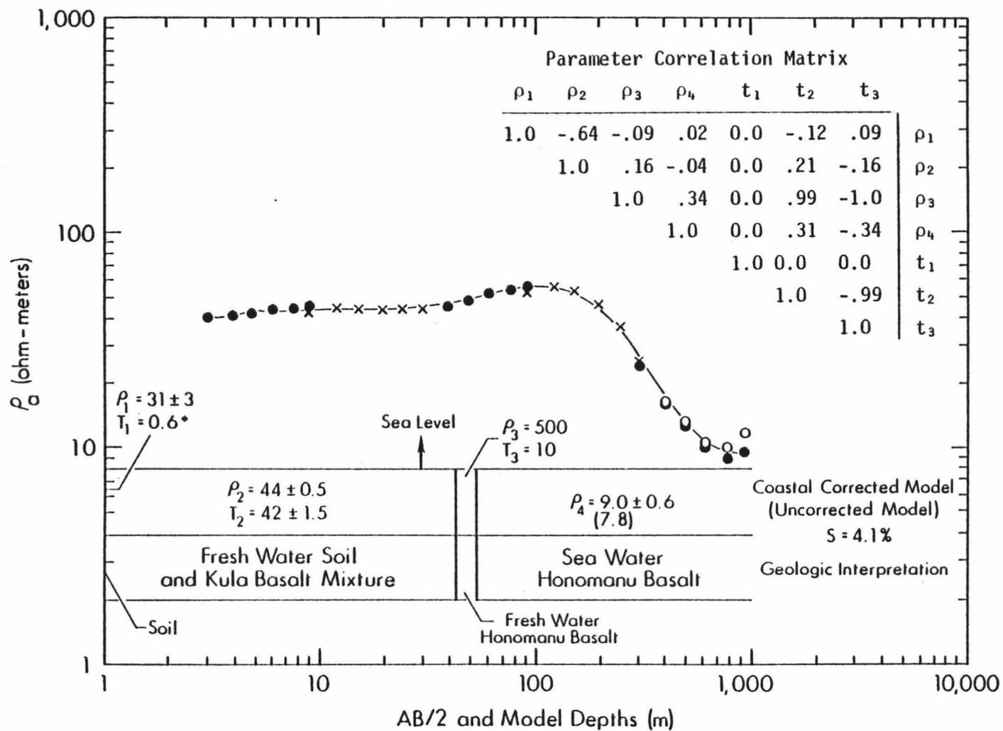
Figure 27. S19 apparent resistivity curve, best fit model and geologic interpretation.
