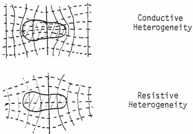
Figure 8. Distortion of potential lines at the earth's surface due to local heterogeneities. Solid lines are equipotentials, dotted lines are current lines. (Modified from Kunetz, 1966, p.13).
