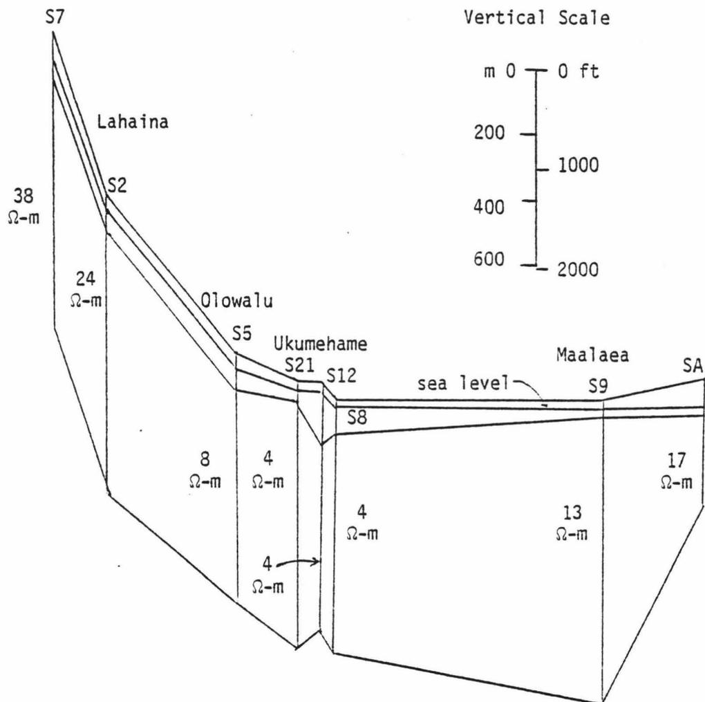
Figure 30. Cross-section of basement resistivities and freshwater lens around the southern coast of West Maui (see Fig. 1). The lowest resistivities are found near Ukumehame valley. All values are interpreted to be seawater-saturated basalt. Vertical exaggeration is 5:1.
