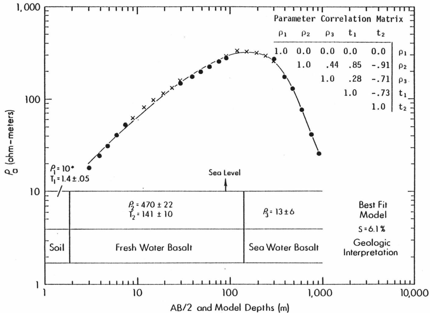
Figure 26. S18 apparent resistivity curve, best fit model and geologic interpretation.
