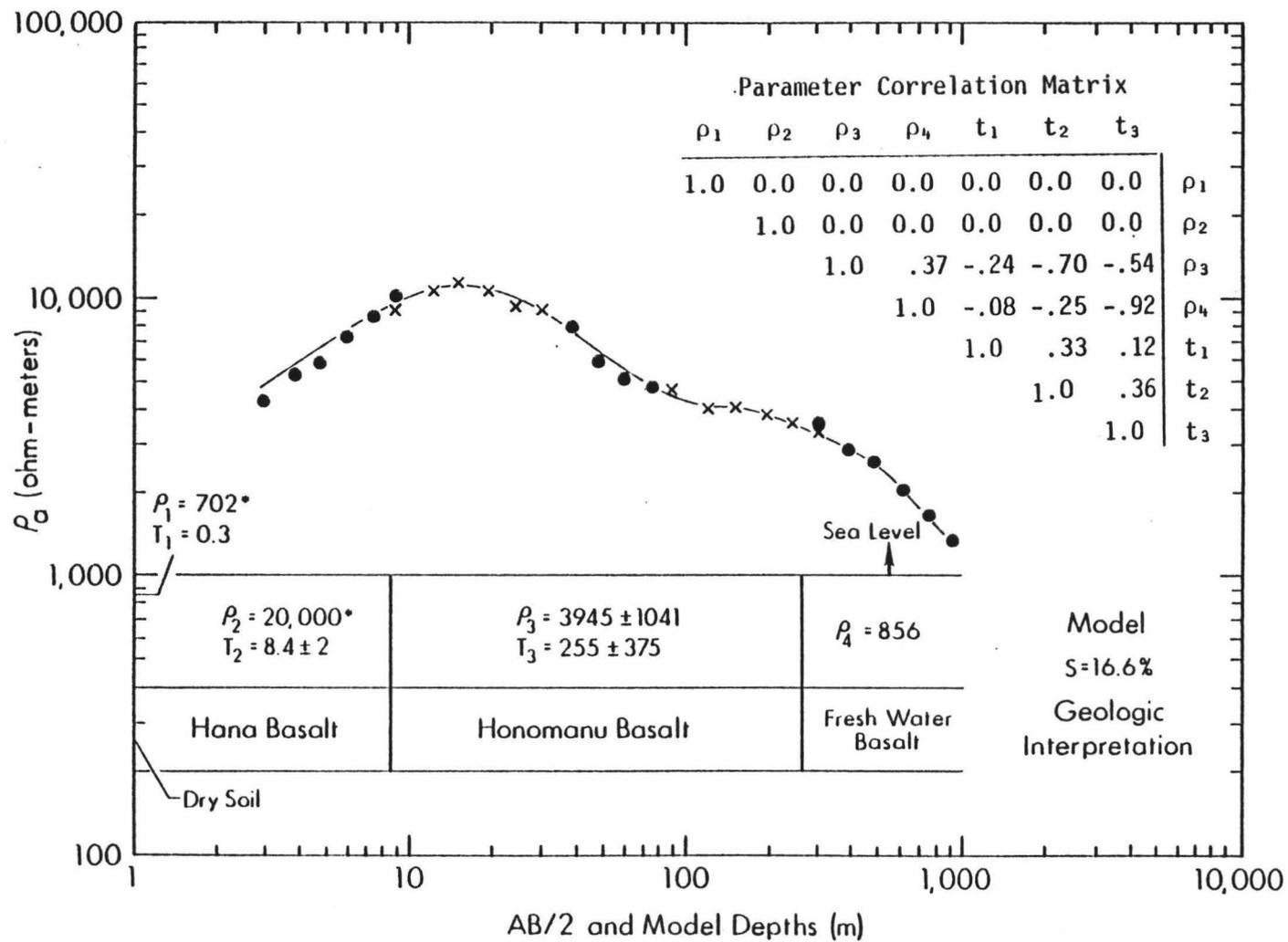
Figure 22. S13 apparent resistivity curve, best fit model and geologic interpretation, note high RMS error (S).
