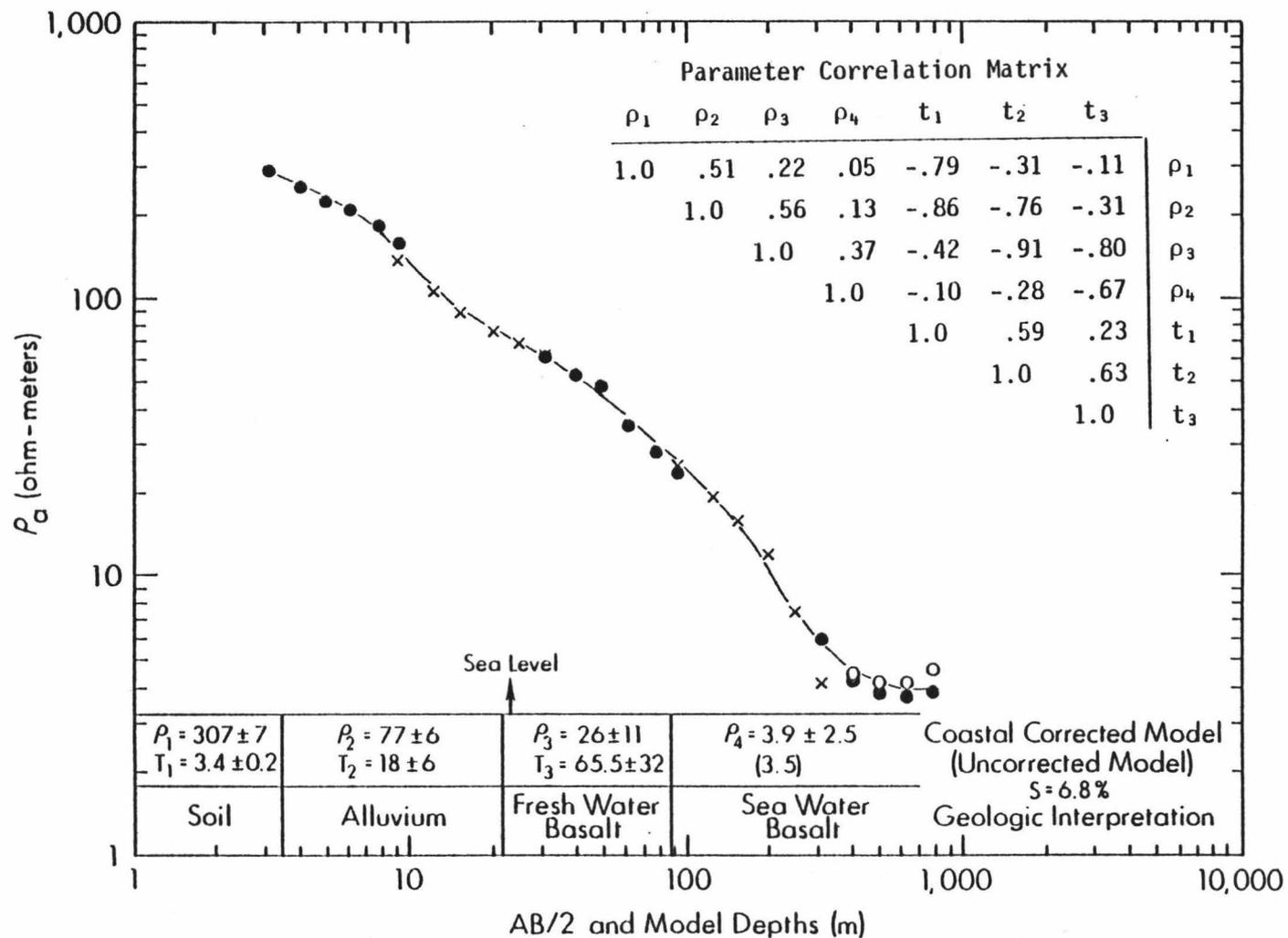
Figure 18. S8 apparent resistivity curve, best fit models and geologic interpretation. The basement resistivity is the lowest measured on Maui.
