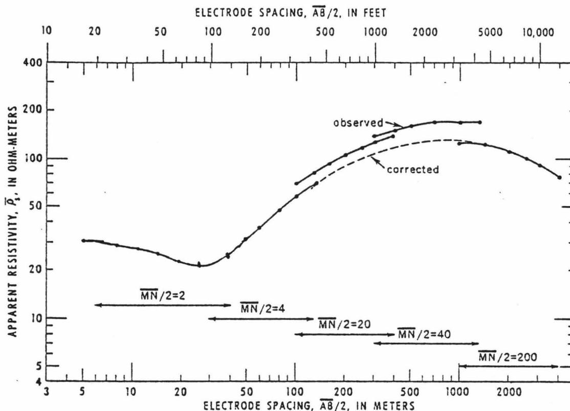
Figure 9. Effect of resistive heterogeneity near potential electrodes at two MN spacings and method of correction. (Modified from Zohdy et al, 1974, p.41).
