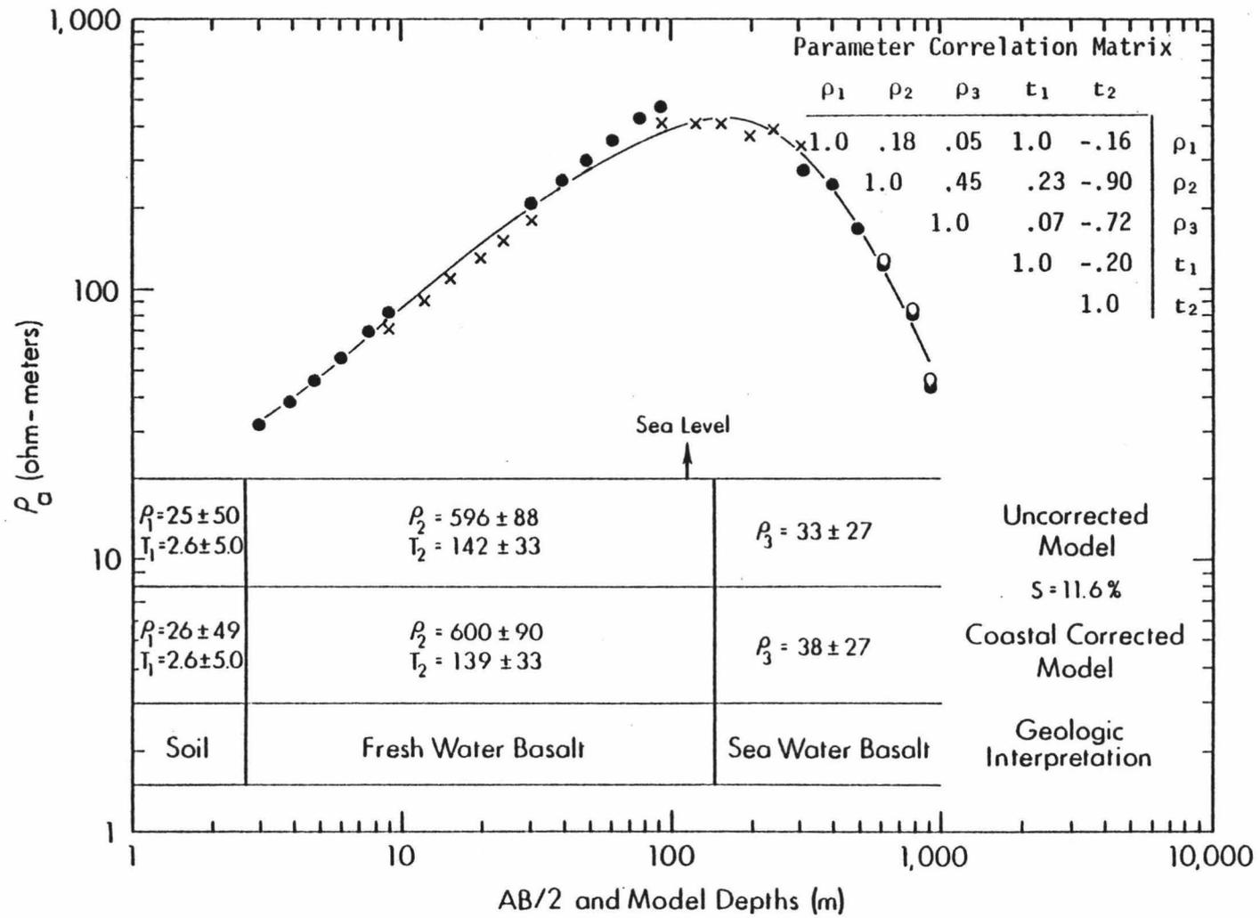
Figure 17. S7 apparent resistivity curve, best fit models and geologic interpretation.
