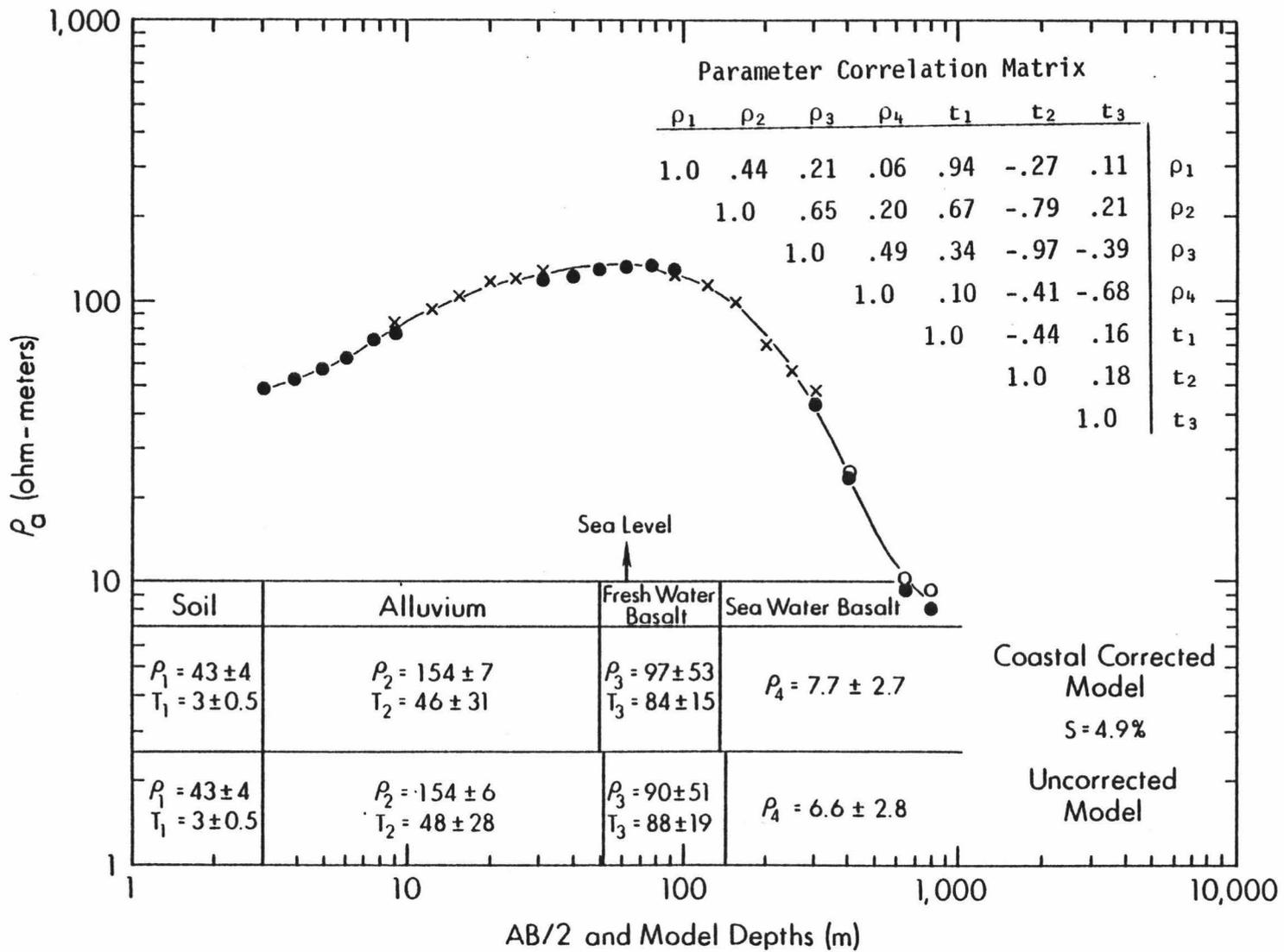
Figure 15. S5 apparent resistivity curve, best fit models and geologic interpretation.
