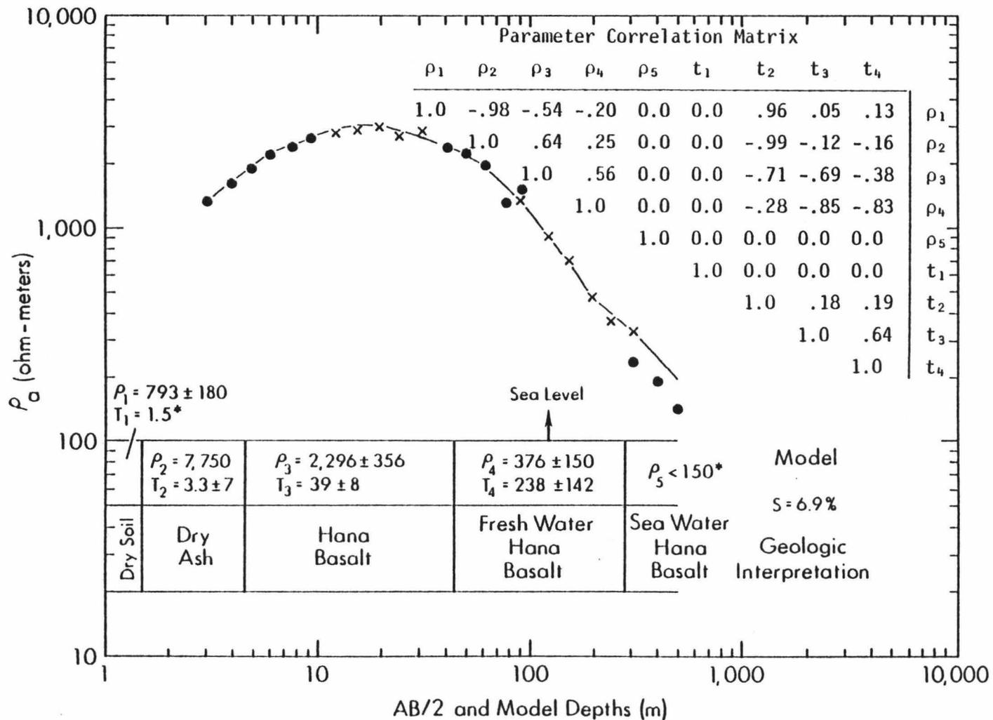
Figure 23. S14 apparent resistivity curve and geologic interpretation. The last 3 data points were shifted upward during the inversion.
