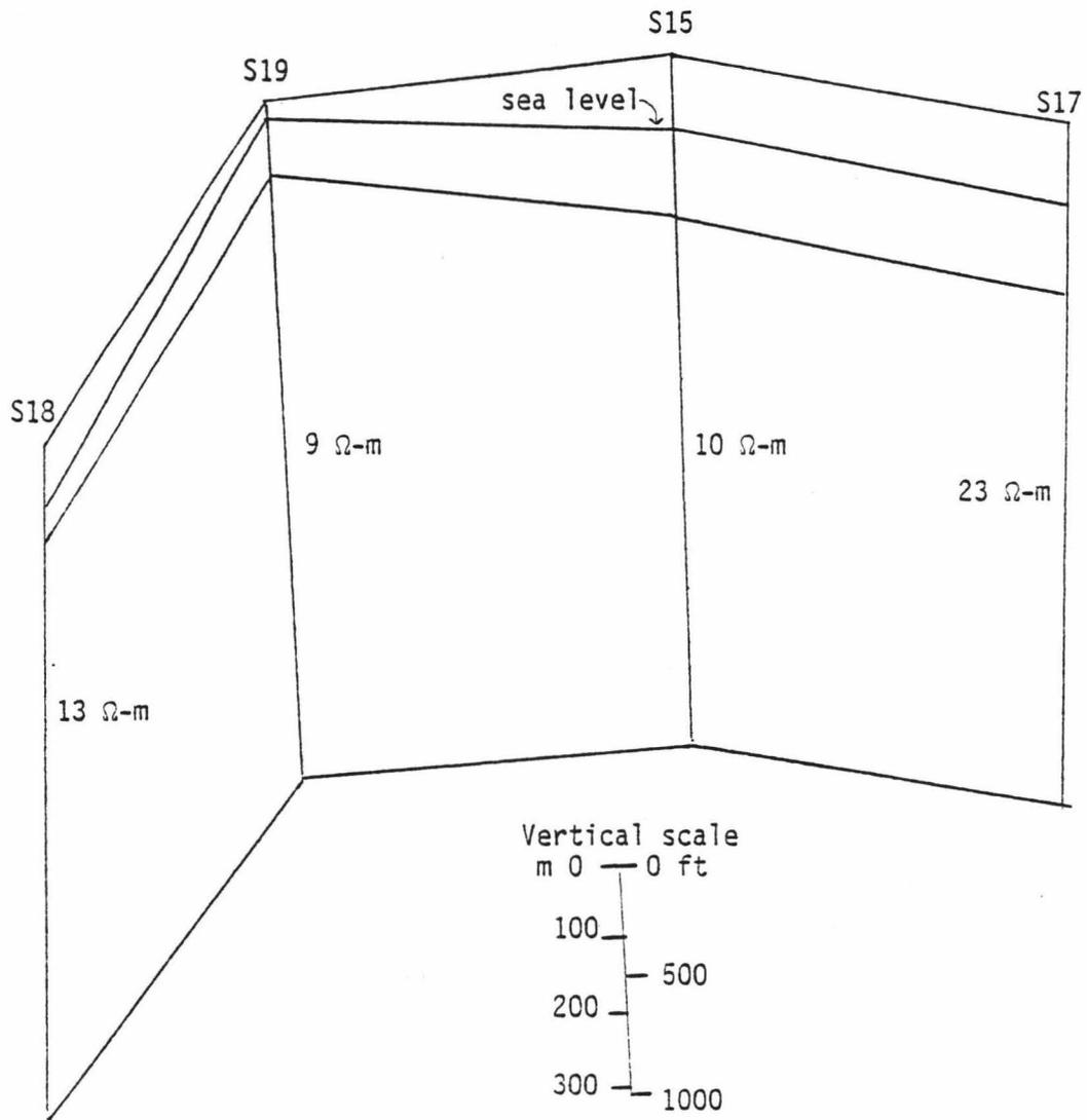
Figure 31. Cross-section of basement resistivities and freshwater lens across the north rift zone of Haleakala. The lowest values correspond with the trace of the rift zone (for locations see Fig. 1). Vertical exaggeration is 10:1.
