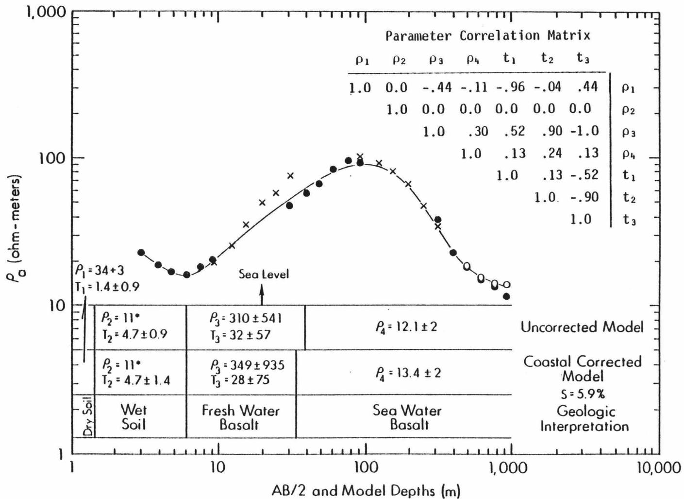
Figure 19. S9 apparent resistivity curve and geologic interpretation. The data from 10 to 30 m AB/2 (x's) were not used during the inversion, see text.
