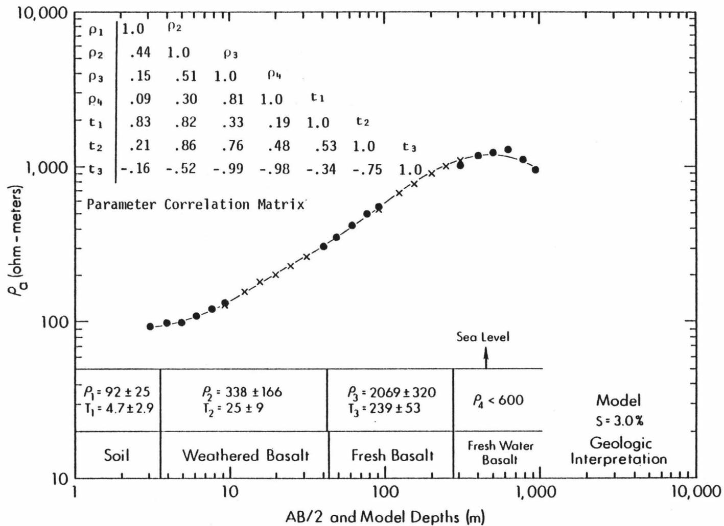
Figure 16. S6 apparent resistivity curve, best fit model and geologic interpretation.
