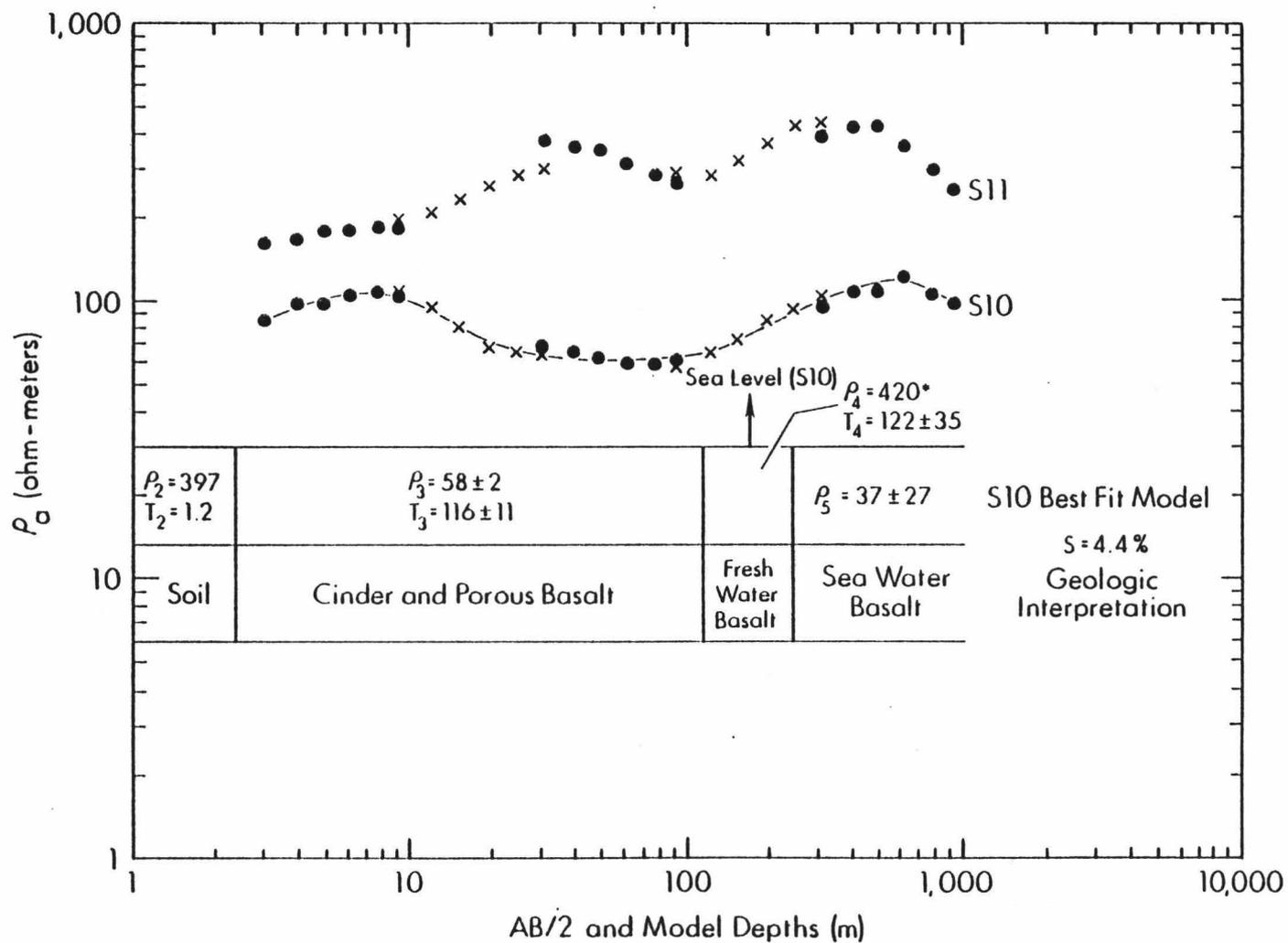
Figure 20. Apparent resistivity curves for S10 and S11, The best fit model and geologic interpretation is given for S10 only, for explanation see text.
