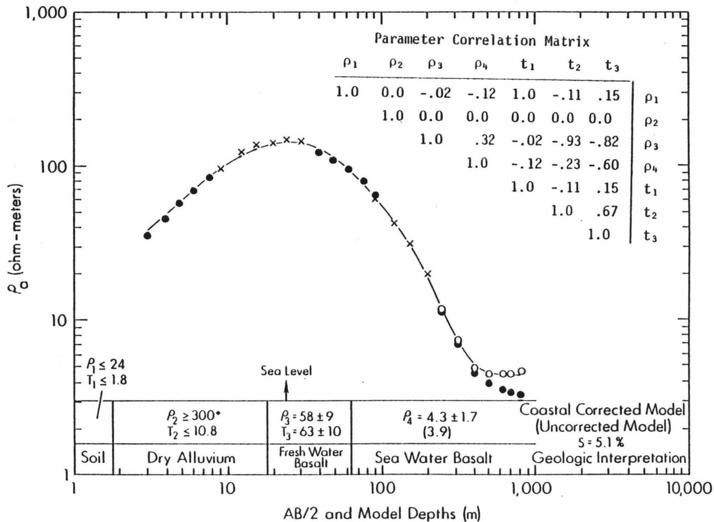
Figure 29. S21 apparent resistivity curve, best fit models and geologic interpretation. Note how application of the coastal correction flattens out the end of the curve.
