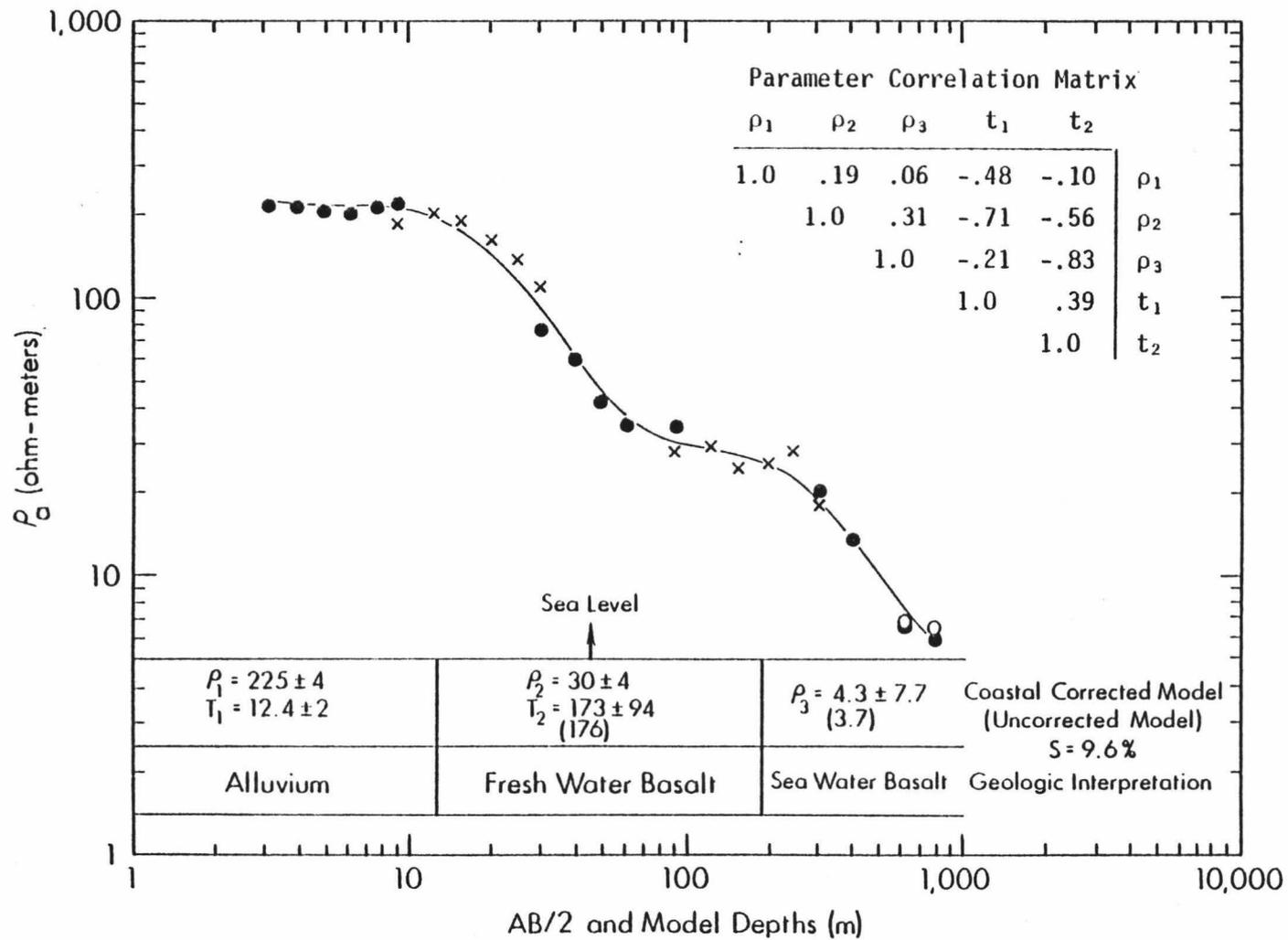
Figure 21. S12 apparent resistivity curve, best fit models and geologic interpretation, note the conductive basement.
