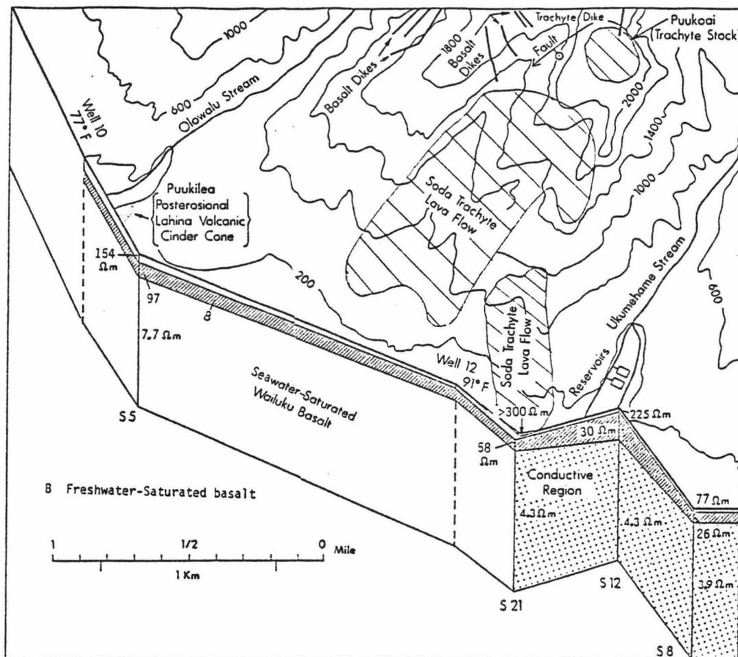
Figure 32. Geoelectric cross-section A'B' across Ukumehame canyon (see fig. 1). Vertical scale equals horizontal scale. The conductive region is interpreted as warm seawater saturating Wailuku basalt.
