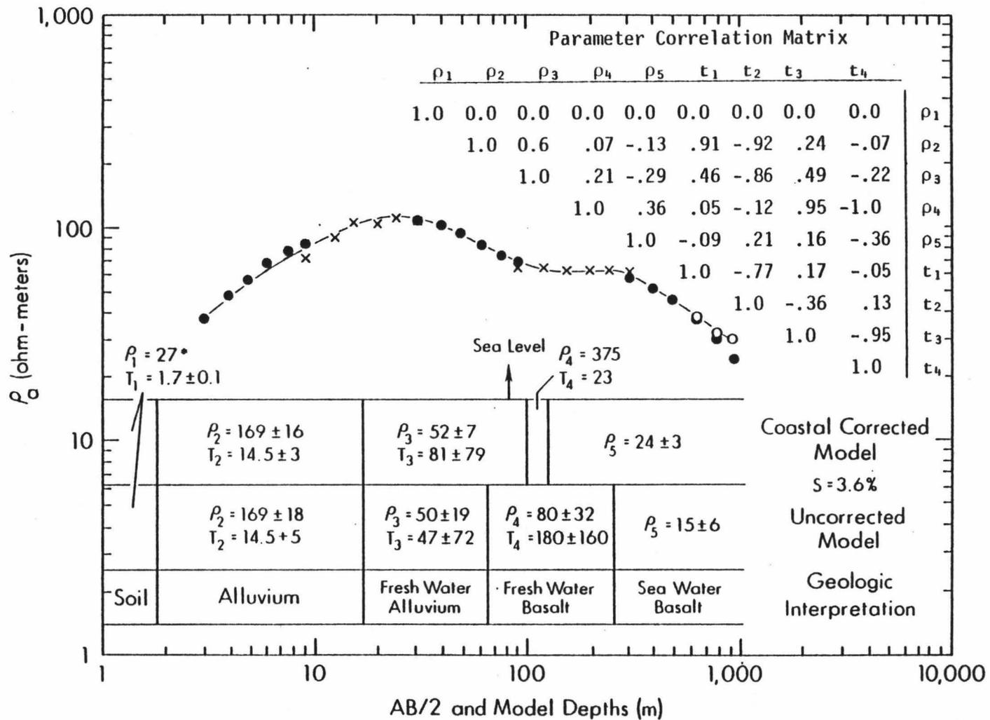
Figure 12. S2 apparent resistivity curve and best fitting models. Note the large parameter changes for layer 4 between the corrected and uncorrected models.
