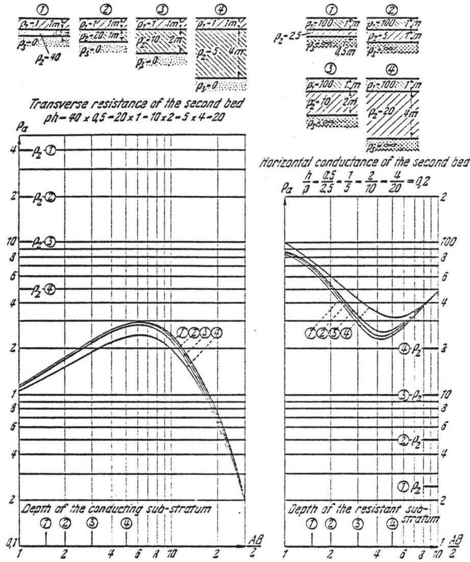
Figure 7. Principle of suppression,  $h$  = thickness and  $\rho$  = resistivity. (Reproduced from Kunetz, 1966, p. 60).
