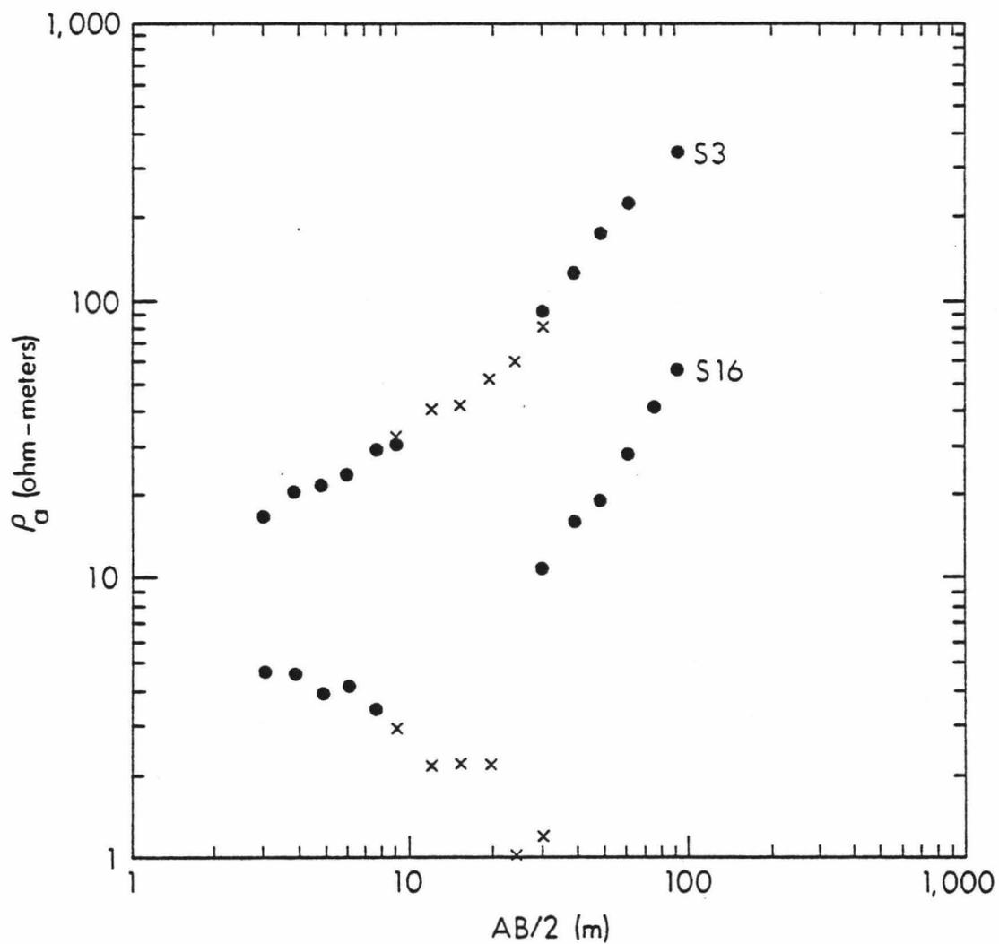
Figure 13. Apparent resistivity curves for S3 and S16. Both curves show the effect of a conductor (water pipe) running parallel to the electrode spread.
