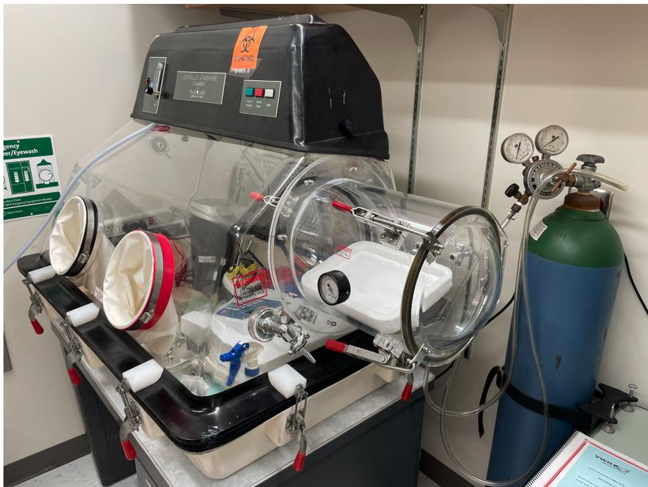
*Figure 6: Controlled atmosphere chamber set up for anaerobic conditions and experimentation under nitrogen gas.*
