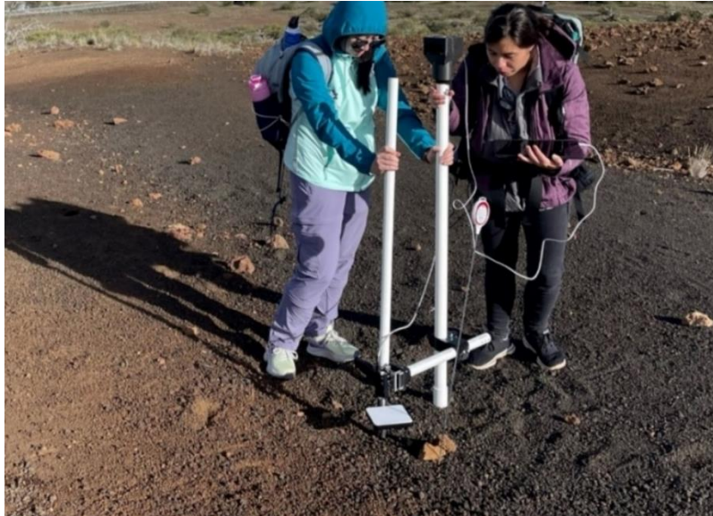
Figure 9: Operators conduct white reference calibration before sampling a spot with strong variations in color in the location between two cinder cones
