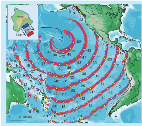
Computer simulation of the tsunami waves that might be set off in a collapse of Kilauea's southeast flank
