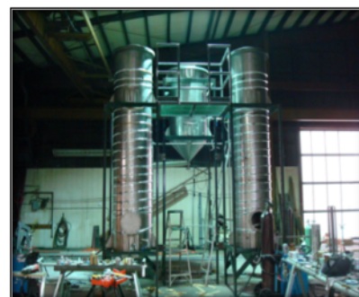
Demonstration reactors under construction, Pacific Biodiesel waste trap grease processing facility.
