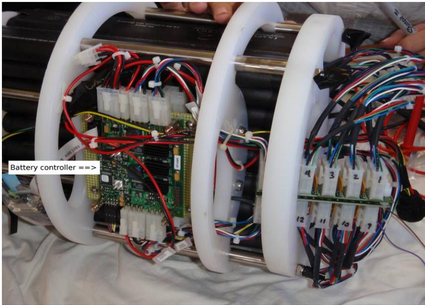
Figure 1.--Battery Controller.
