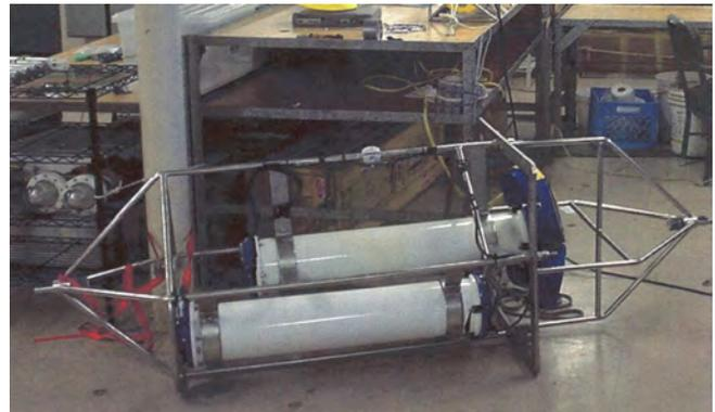
**FIGURE 4:** RDI 75 kHz ADCP just after recovery from a seven month deployment in HOME. The ADCP’s transducers are at the right and face upward when the cage is attached to the mooring line. The second white cylinder in the foreground is an external battery case.
