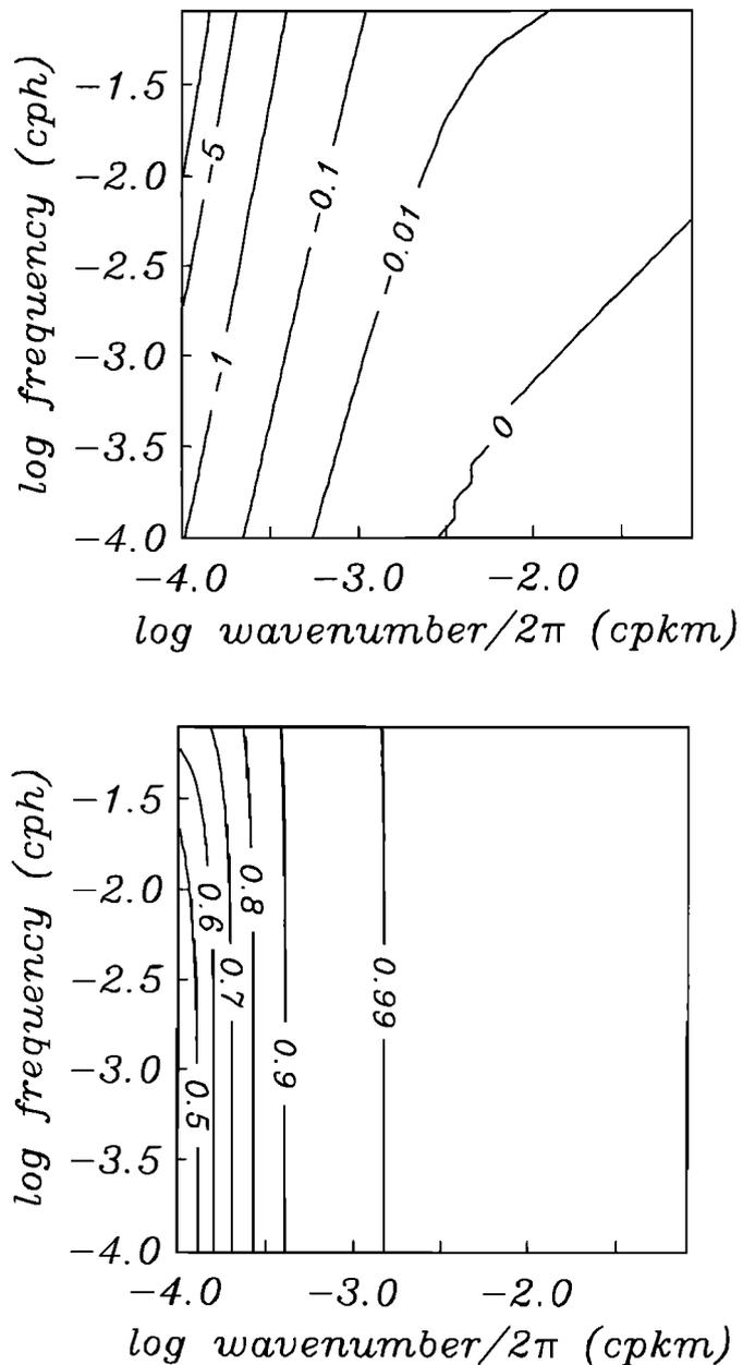
Fig. 4. Contour plots of the magnitude (bottom) and phase in degrees (top) of  $\Gamma$  given by (53) in the text as a function of frequency and inverse wavelength using the Pacific reference model of Figure 3.
