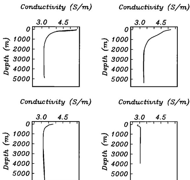
Fig. 10. Conductivity profiles computed using the empirical formulae of *Fofonoff and Millard* [1983] with zonally averaged salinity and potential temperature (converted to in situ temperature) data from *Levitus* [1982]. The locations shown are 12.5°N Pacific (upper left), 32.5°N Atlantic (upper right), 42.5°N Pacific (lower left), and 57.5°S Atlantic (lower right). The expansions of these profiles in horizontal velocity structure functions are listed in Table 1.
