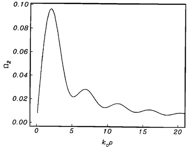
Fig. 8. Approximate form of the horizontal electric field averaging kernel given by (57) in the text divided by the angular factor  $\nabla_h \rho$ . The abscissa shows horizontal distance in units of  $k_i^{-1}$  which is of order units of water depths.
