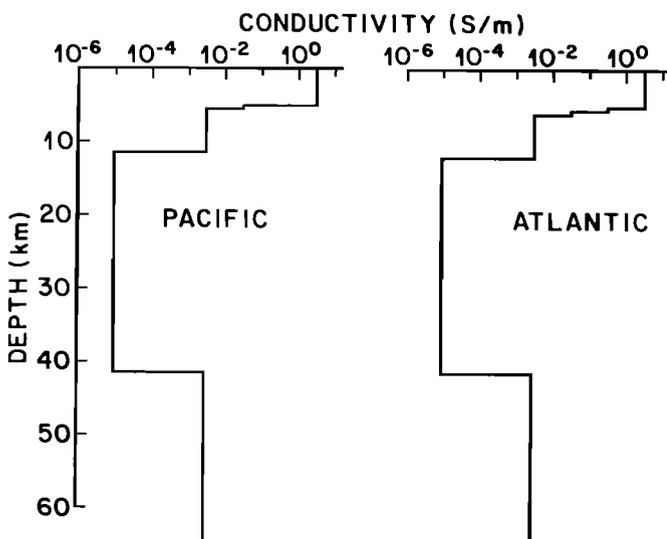
Fig. 3. The Pacific (left) and Atlantic (right) reference models for the conductivity structure beneath the ocean as given by *Chave et al.* [1990]. The two differ by the presence of a thin ( $\approx 0.5$  km) layer of relatively conductive sediment in the Atlantic model. Both models are terminated in a half-space of conductivity 0.1 S/m below 71 km depth.
