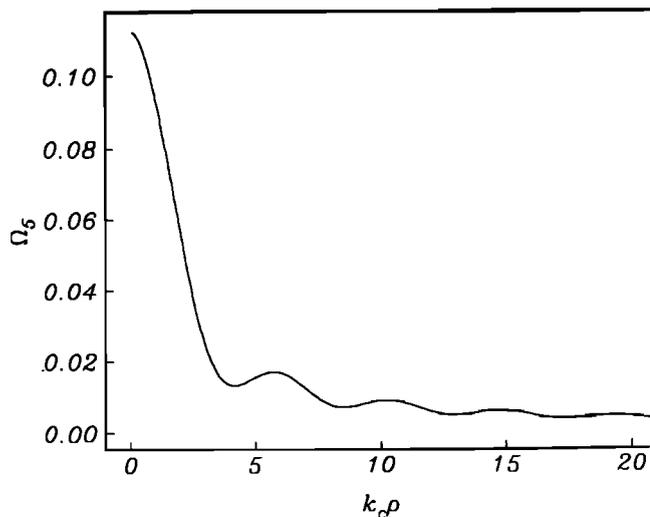
Fig. 9. Approximate form of the vertical magnetic field averaging kernel given by (60) in the text. The abscissa shows horizontal distance in units of  $k_c^{-1}$  which is of order units of water depths.
