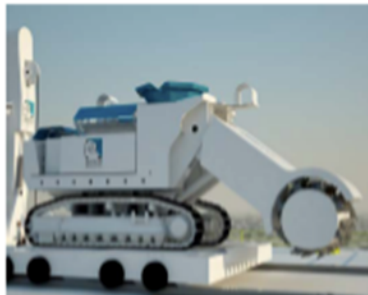
Bulk Miner – cuts ore at high rates on areas benched by Auxiliary Miner
