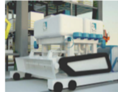
Gathering Machine – slurries cut ore with seawater and transfers to RALS
