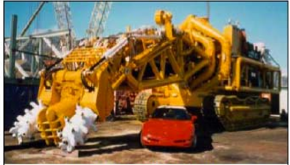
Second generation 200 ton offshore diamond mining machine, DeBeers, Namibia Courtesy Marine Minerals Pty
