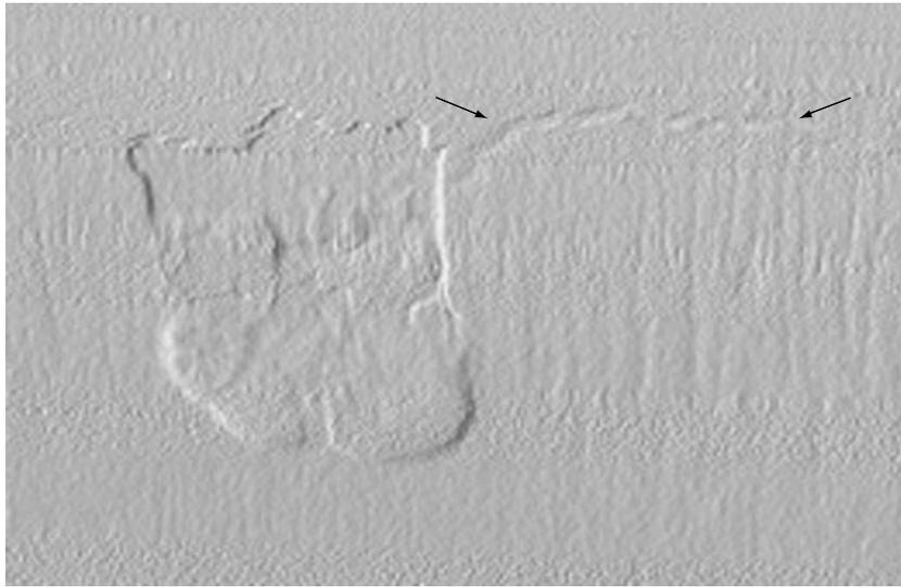
Fig. 17. Sidescan sonar image of a submarine landslide off the coast of Santa Barbara, California (courtesy of the Monterey Bay Area Aquarium Research Institute). The view is to the east. To the north (left) of the slide the slope appears undeformed. To the south (right) of the slide is a fracture about 4 km long, marked by arrows. This is interpreted to represent fracturing produced in an incipient stage of sliding and to mark the future location of a head scarp.
