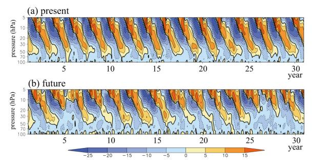
Zonal-mean zonal wind over the equator for (a) present day and (b) double  $CO_2$  conditions. Results shown for pressures between 100 and 5 hPa corresponding to heights of about 17 to 35 km. The color bar is labeled in m/s and the contour interval is 5 m/s.
