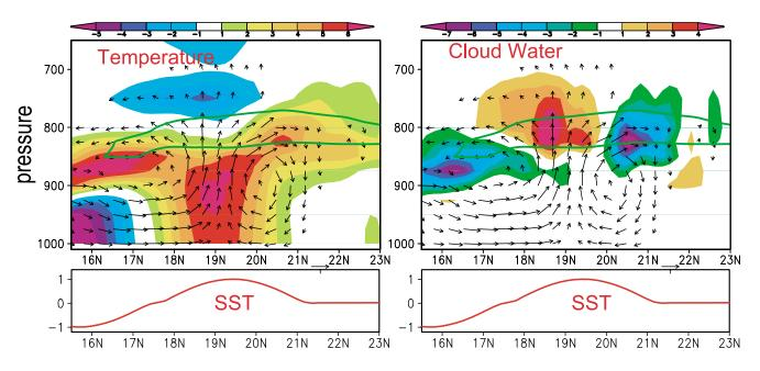
**Figure 1:** Latitude-pressure sections of temperature (upper left) and cloud-water content (upper right). Superimposed are meridional circulation anomalies of the Hawaiian wake simulated in a regional atmospheric model. The SST anomalies taken from satellite measurements (plotted in duplicate in lower panels) are imposed uniformly in the zonal direction west of Hawai'i.
