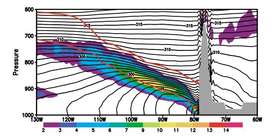
**Figure 5**: Vertical structure of the simulated stratus-cloud deck at 10°S in the southeastern equatorial Pacific: cloud-water content (color shade:  $10^{-2}$ g/kg) and virtual potential temperature (black contours, in °K) averaged for August–October, 1999. The dθ<sub>V</sub>/dp = 8 °K/100hPa (red curves) marks the mean location of the inversion layer that caps the planetary boundary layer. Note that both the inversion and cloud layer increase in height west of the Andes (gray shaded).
