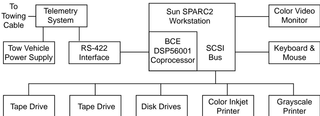
Figure 3. Schematic diagram of HAWAII MR1 surface electronics.
