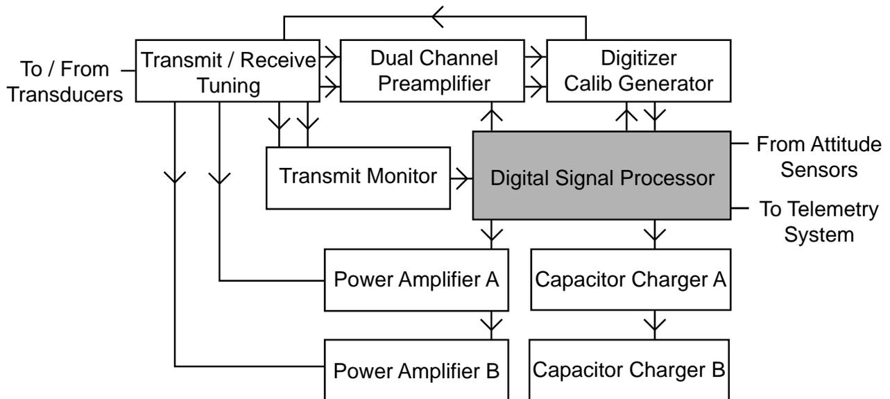
**Figure 2.** Schematic diagram of subsurface electronics for HAWAII MR1. Drawing illustrates one side only; electronics are identical on both port and starboard sides. Each block represents a single printed circuit board.
