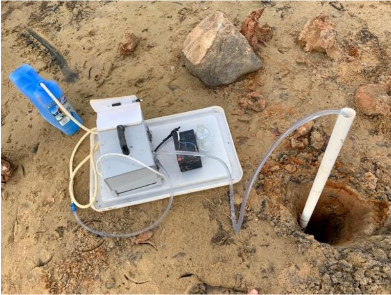
Fig. S1.4. Photo of sampling from a groundwater well using a peristaltic pump.
