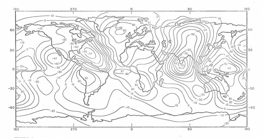
FIGURE 1. GEOIDAL UNDULATIONS IN METERS REFERRED TO AN ELLIPSOID WHOSE  $C_{20}$  COEFFICIENTS COINCIDE WITH THE SATELLITE-OBSERVED ONES. COMPUTED USING MEAN ZONALS AND TESSERALS UP TO  $P_{88}$  AS DEFINED IN THE TEXT. CONTOUR INTERVAL: 10 METERS
