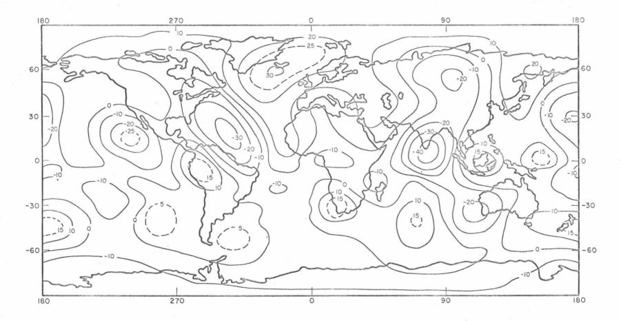
FIGURE 5. GRAVITY ANOMALIES IN MILLIGALS REFERRED TO THE INTERNATIONAL GRAVITY FORMULA. COMPUTED USING MEAN ZONALS AND TESSERALS UP TO P<sub>88</sub> AS DEFINED IN THE TEXT. CONTOUR INTERVAL BETWEEN SOLID LINES: 10 MILLIGALS; BETWEEN SOLID AND BROKEN LINES: 5 MILLIGALS
