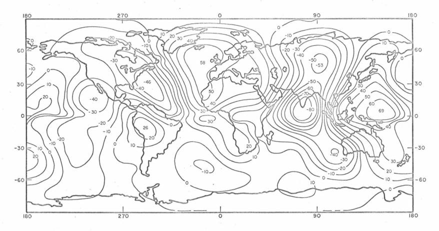
FIGURE 3. GEOIDAL UNDULATIONS IN METERS REFERRED TO A BEST-FITTING SATELLITE SPHEROID AS DEFINED IN THE TEXT. COMPUTED USING MEAN TESSERAL COEFFICIENTS UP TO P<sub>88</sub> AS DEFINED IN THE TEXT.
