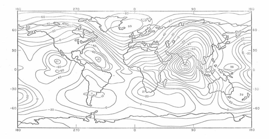
FIGURE 2. GEOIDAL UNDULATIONS IN METERS REFERRED TO THE INTERNATIONAL REFERENCE ELLIPSOID. COMPUTED USING MEAN COEFFICIENTS UP TO P<sub>88</sub> AS DEFINED IN THE TEXT.
