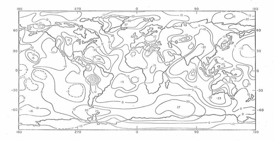
FIGURE 6. GRAVITY ANOMALIES IN MILLIGALS (TAKEN FROM KAULA, 1966). RESULTS COMBINE AVAILABLE SURFACE GRAVITY MEASUREMENTS WITH SATELLITE INFORMATION. CONTOUR INTERVAL BETWEEN SOLID LINES: 10 MILLIGALS; BETWEEN SOLID AND BROKEN LINES: 5 MILLIGALS
