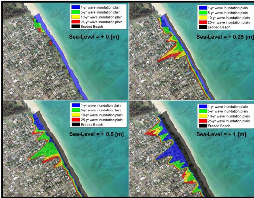
Figure 6 - Illustrating approach #2 - inundation contours for different scenarios of sea-level rise [0 (at present time), +0.25 (2025), +0.5 (2050), +1.0 m (2100)], and an eroded beach contour from a constant erosion rate of 0.6 m/yr.
