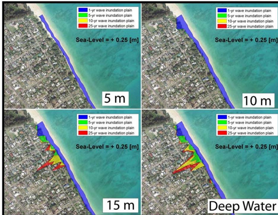
Figure 7 - Illustrating approach #3 - Projected inundation lines under a scenario of +0.25 m of sea-level rise with the runup computed from wave heights at different depths (5 m, 10 m, 15 m, and from deep water). The reverse shoaling and dissipation on the reef face is responsible for the significant reduction in runup and inundation at the coast.
