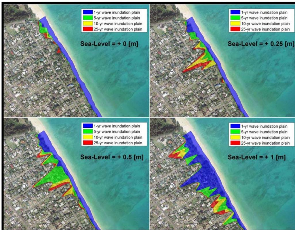
**Figure 5** - Illustrating approach #1 - inundation contours for different scenarios of sea-level rise (0, +0.25, +0.5, +1.0 m).
