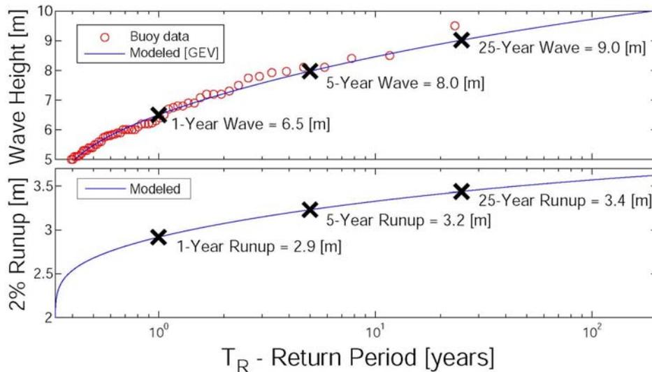
Figure 4 - Return significant wave height [m] and return period [years] for Waimanalo for the northeast swell window 75-35° (Top) and corresponding return runup elevation [m] and return period [years] (Bottom) given by the Stockdon (2006) empirical runup relation using a nominal wave period of 16 sec. and a beach slope 1/24.
