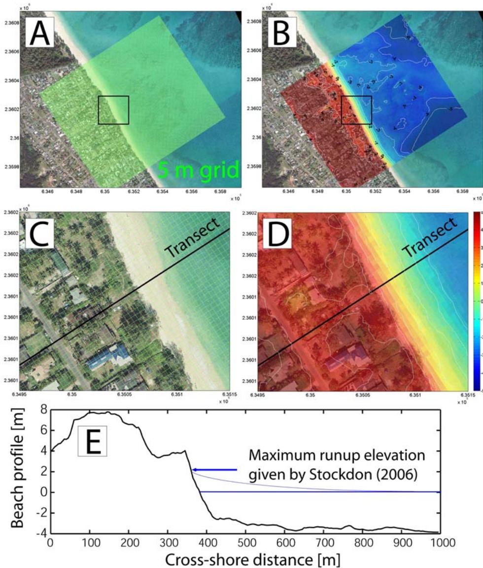
Figure 2 – The Waimanalo runup grid (A) and elevation (B) from a broad view. Beach profiles (E) are extracted from transects along shore-normal grid lines (C) where the elevation is given by a LIDAR survey (D).
