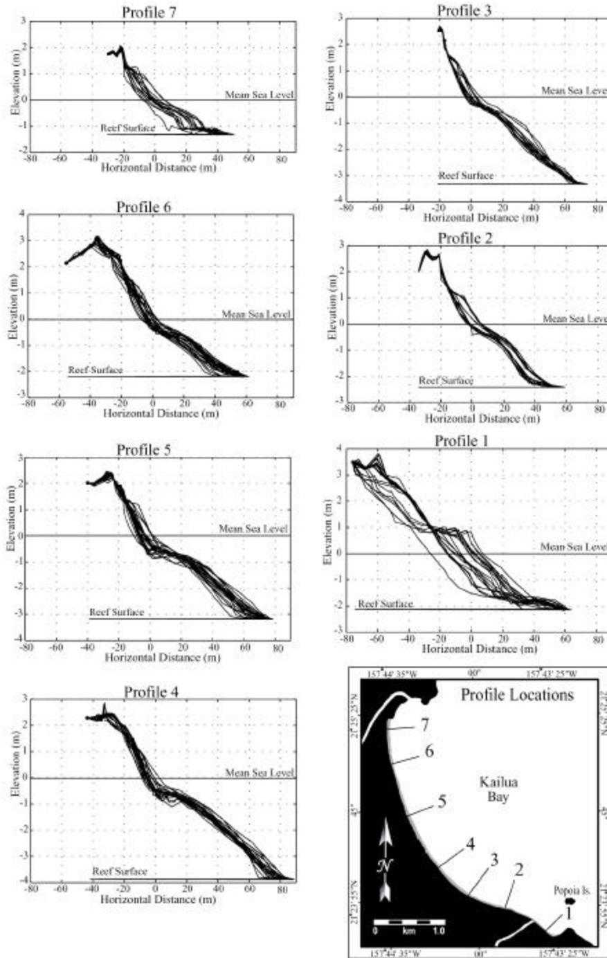
Figure 2. Kailua Beach, Oahu, profiles demonstrate the variability in sand volume and depth of the fringing reef along the length of the bay.
