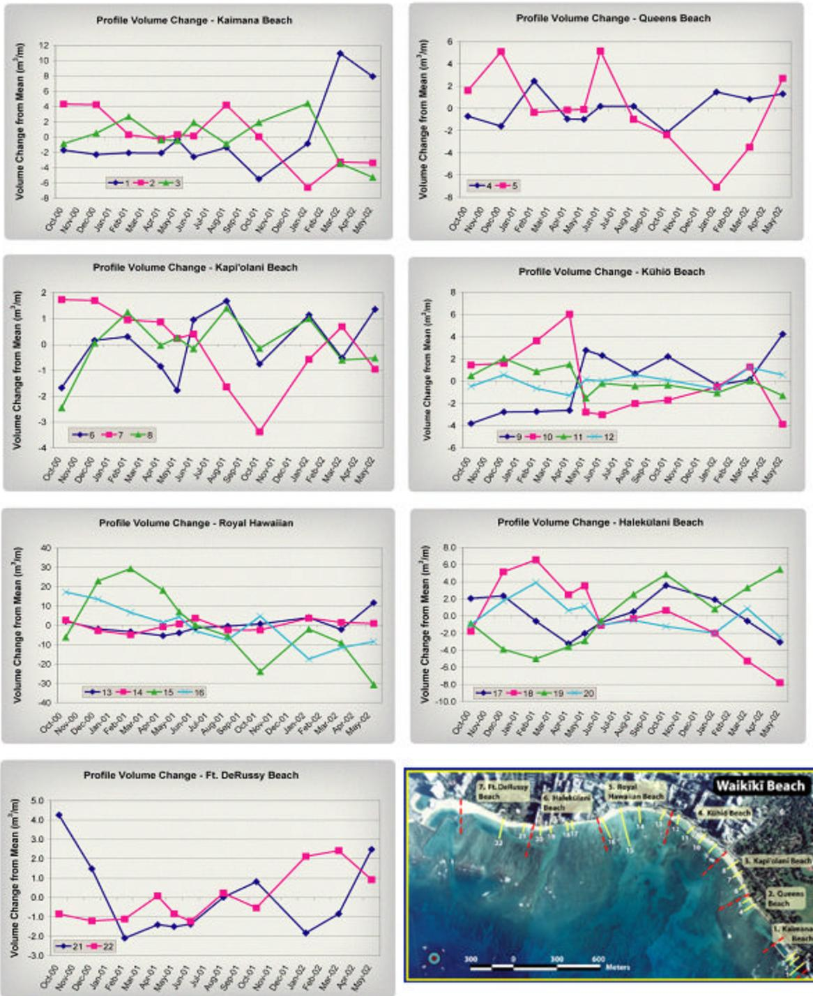
Figure 4. Beach profile volume changes at Waikiki, Oahu, relative to the mean, for 22 profiles in 7 littoral cells (Miller, 2002). Note the opposing inflation/deflation occurring at neighboring profiles in a given cell.
