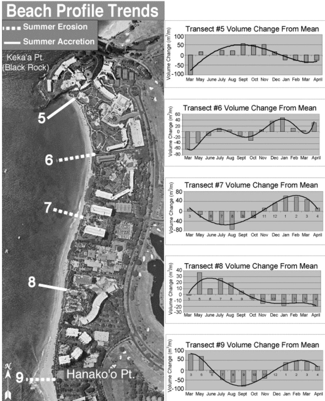
Figure 5. Beach profile trends at Kaanapali, Maui, with alternating patterns of erosion and accretion demonstrated on the photomosaic by solid versus dashed lines. Volume plots to the right reveal the cyclic nature of the profiles as seen by the best fit trend line (Eversole, 2002).
