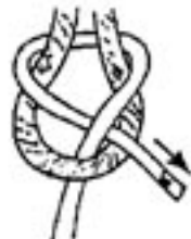
Sheet bend: start with a loop
