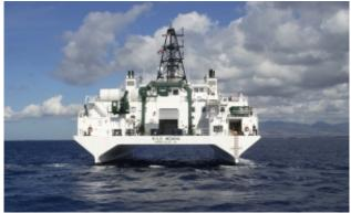
Kilo Moana is the newest research vessel in the UNOLS fleet. The ship's unique SWATH design makes Kilo Moana an ideal seafloor mapping vessel.
