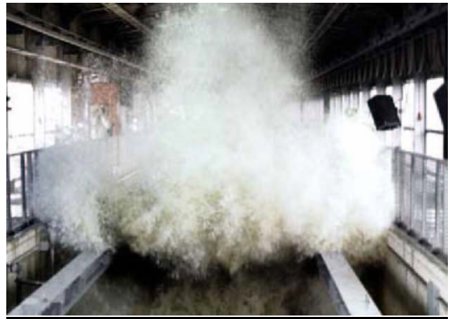
Figure 7. Extreme wave reproduced in the Hannover wave tank.
