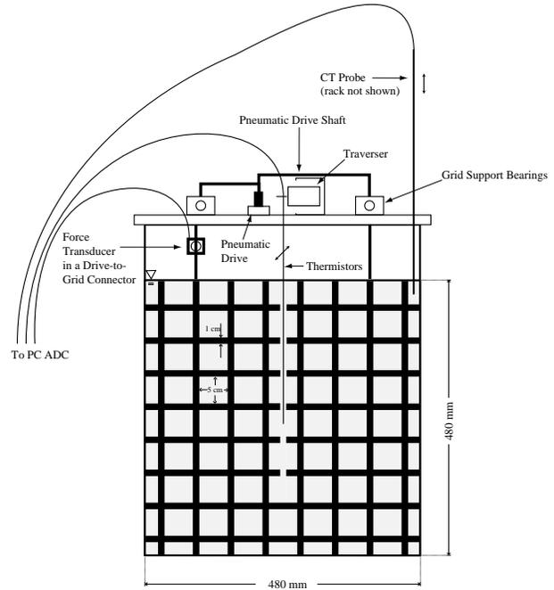
**Figure 1.** Schematic diagram of the front view of the experimental setup. The tank is 520 mm long, and was filled with a linearly salt stratified fluid. The vertical rigid grid stirred the entire fluid volume.
