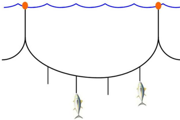
**Fig. 3** Depiction of a pelagic longline, whereby mainline is suspended by a series of floats, with baited hooks at terminal ends of the gangions
