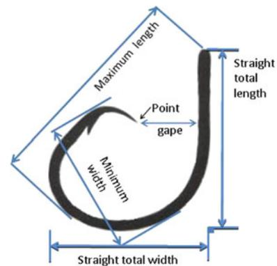
**Fig. 1** Dimensional terms of a circle hook (adapted by Yokota and Boggs, pers. comm.)
