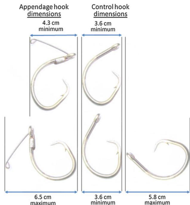
**Fig. 2** 14/0 circle hook with appendage and standard control 14/0 circle hook
