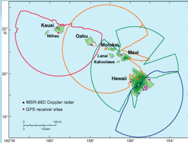
Four radars provide rain rates and wind data for near vicinity of Hawaii. Important for nowcasting of thunderstorms and flooding.
