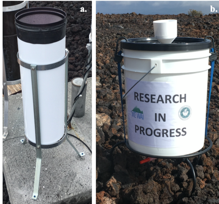
Figure 2.2. Precipitation collector designs. (a) A NovaLynx Rain and Snow Gauge, deployed at the Mauna Loa Observatory. (b) A bucket-style rain collector, deployed at Humu‘ula.
