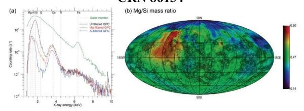
A solar flare solar monitor (SAX) spectrum, corresponding Gas Proportional Counter (GPC) X-ray spectra of filtered and unfiltered detectors, and a final data product Mg/Si map of Mercury as obtained by MESSENGER are presented side by side. The two endpoint products, recorded spectra and global elemental abundance (elemental ratio) maps illuminate sophistication and success in elemental mapping with planetary X-ray fluorescence spectrometry.
