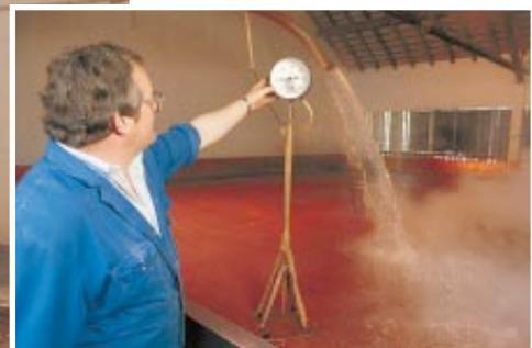
When the long boil is done, the liquid is pumped into a cooling tun in the brewery’s attic (left). This is the unique, signature event in the creation of lambic, when local microflora, including wild yeasts, inoculate the brew. Fans circulate the air while the liquid’s temperature drops to about 15 degrees Celsius (above).
