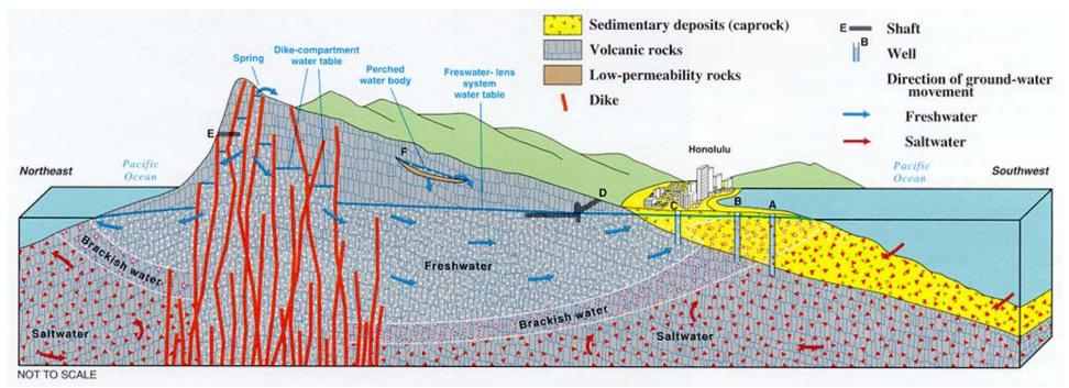
Figure 1. schematic cross section of the island of Oahu showing various hydrogeological features and different water development installations (Gingerich and Oki, 2000).
